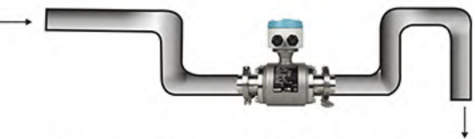
Install at the lowest point when used in open drain pipe
