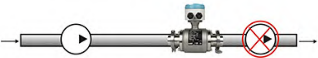
Don't install it at the entrance of pump, install it at the exit of pump
