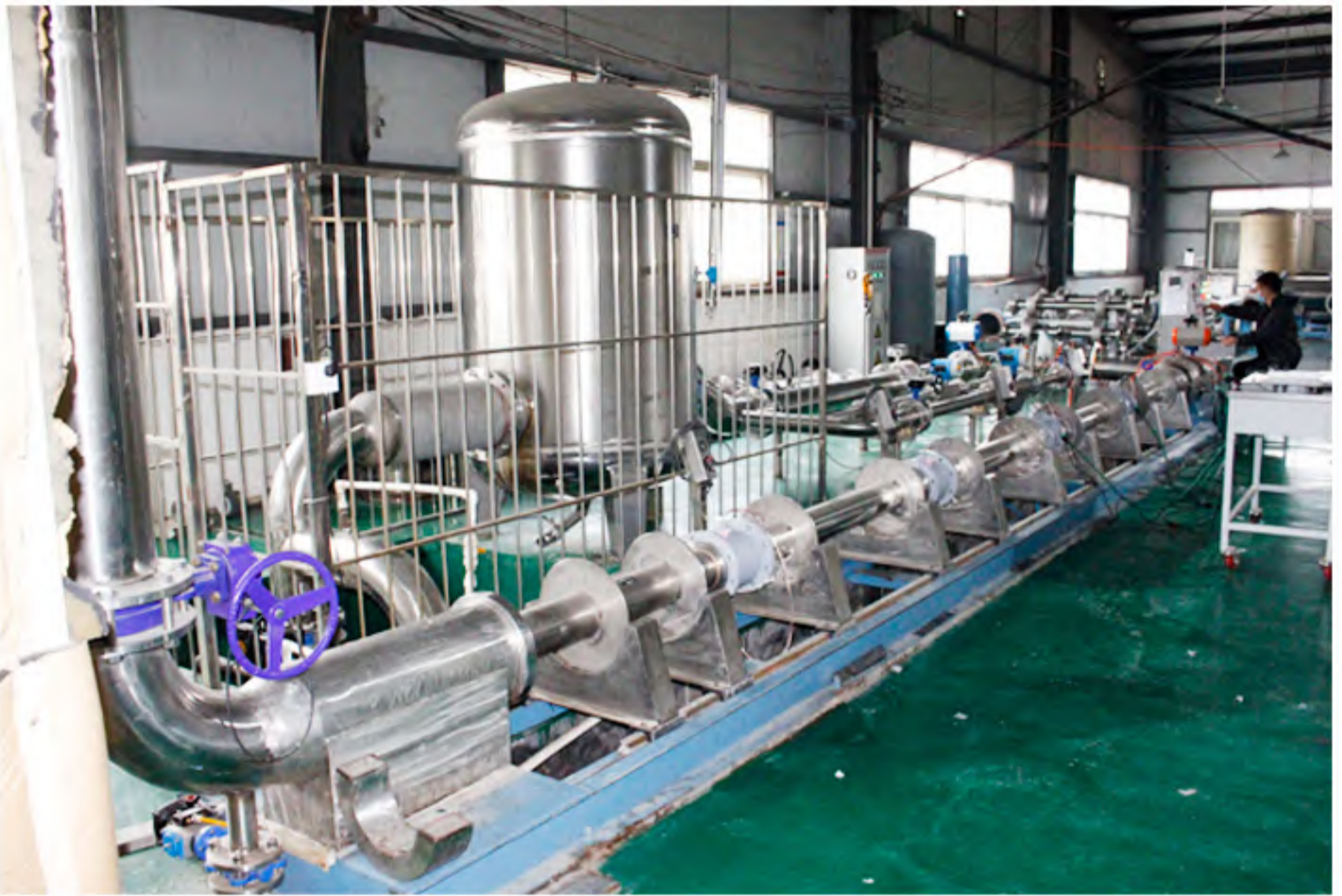
DN65-DN300 Gravimetric & Standard Meter Liquid Flow Meter Calibration Device
